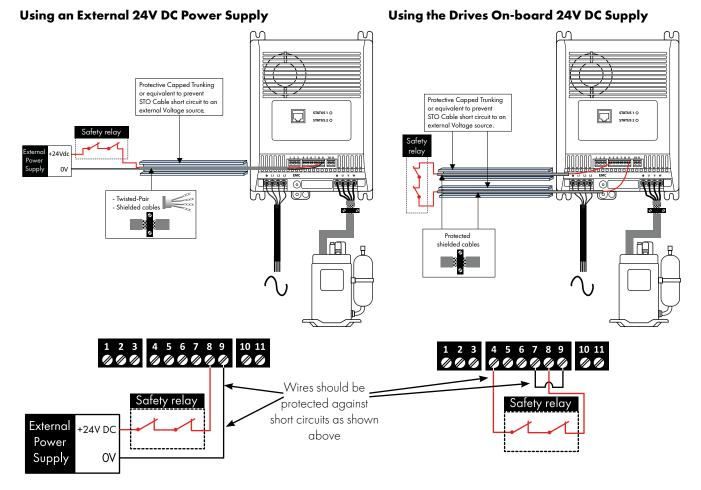
NOTE The Maximum cable length from Voltage source to the drive terminals should not exceed 25 metres.
