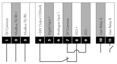
STO signal must be provided in order to permit running the motor. Start/Stop commands and speed reference are provided by serial communication. In Modbus mode, the digital input and analogue input can be used as remote I/O by the controller, the relay output can also be configured to be controlled by Modbus and used by the controller if required.
