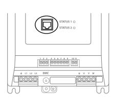
The RJ45 port has some terminals that are internally connected in parallel with the pluggable control terminals as shown below:
