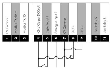
STO signal must be provided in order to permit running the motor. Start/Stop command provided by the Digital Input (P1-11 = 1) or when the analogue input level is greater than 1% (if P1-11 = 2) and speed reference provided by the Analogue input.
